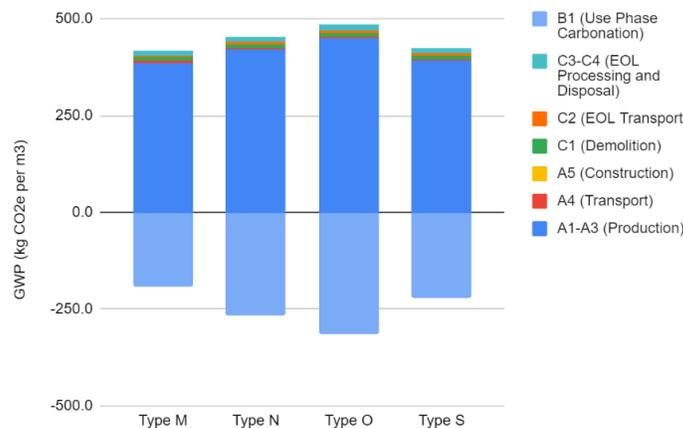
Figure 5. GWP per metric ton for four mortar types.
