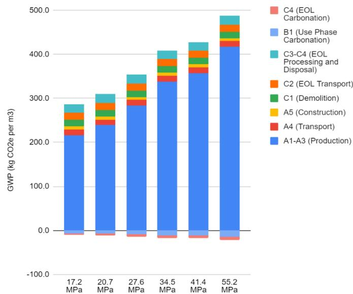
Figure 3. GWP per m3 for ready-mix concrete of six strength classes.
