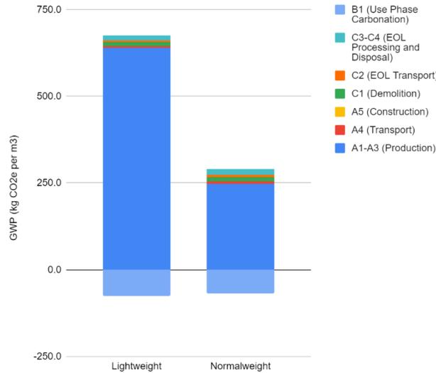
Figure 4. GWP per metric ton for normal-weight and lightweight CMU.
