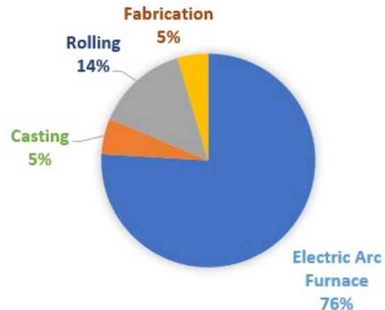
**Figure 3. Relative comparison of average carbon intensity of processes in 100% recycled EAF steel. (Based on percent of kgCO<sub>2e</sub> / ton of steel product.)**
