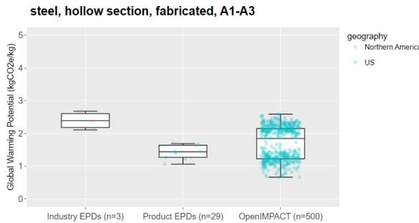
**Figure 6. Comparison boxplot for steel, hollow section, fabricated, A1-A3, North American region.**
