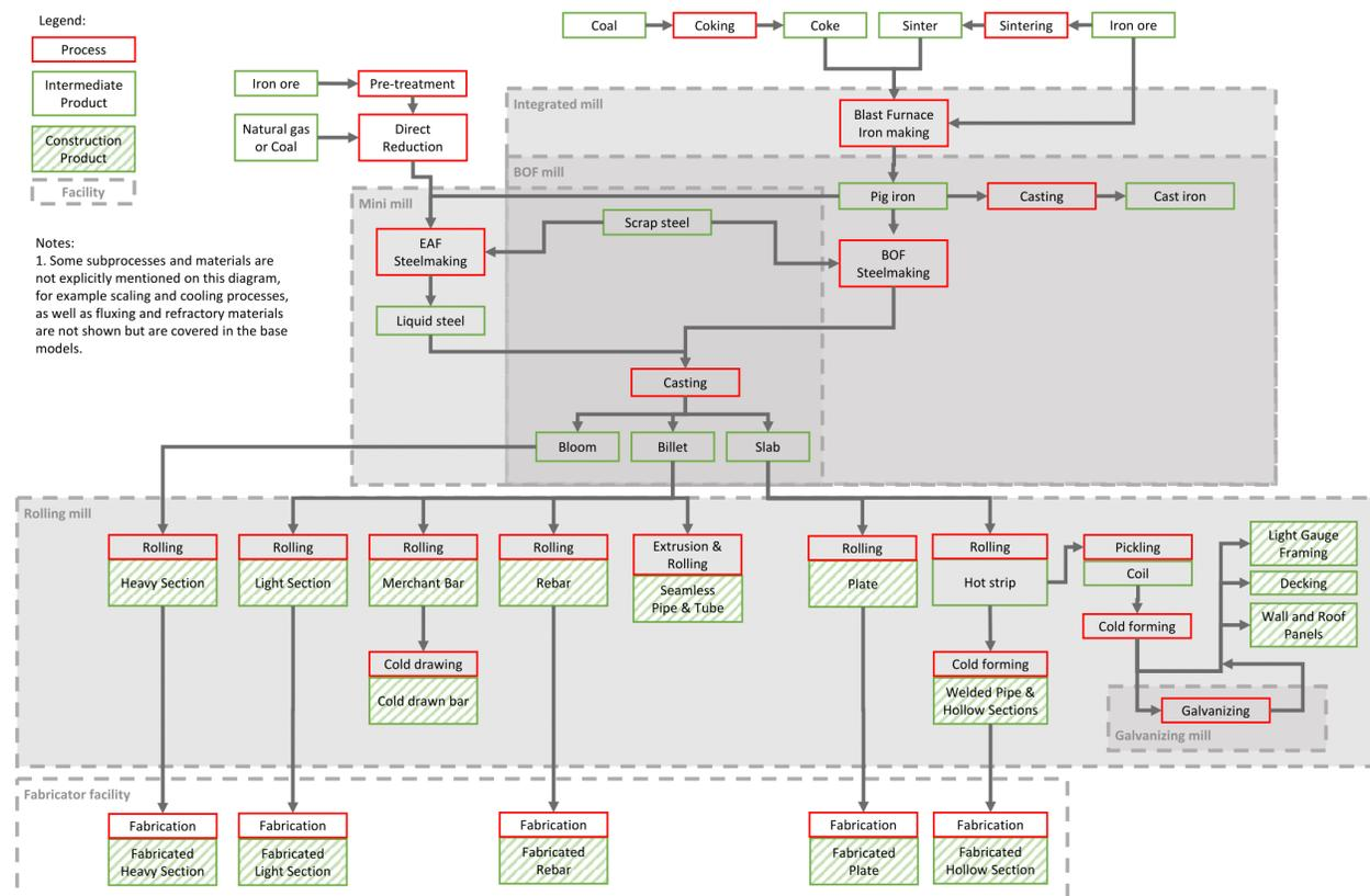
Figure 1. Simplified schematic of the main production routes for steel construction products.
