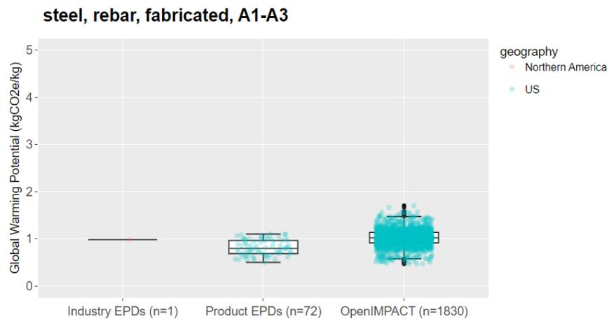
**Figure 10. Comparison boxplot for steel, rebar, fabricated, A1-A3.**
