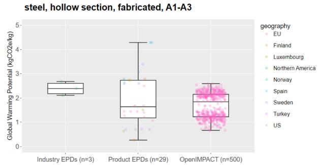
**Figure 7. Comparison boxplot for steel, hollow section, fabricated, A1-A3, all regions.**
