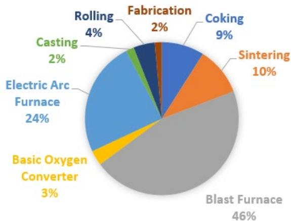
**Figure 2. Relative comparison of average carbon intensity of processes in the production of steel construction products. (Based on percent of kgCO<sub>2e</sub> / ton of steel product.)**
